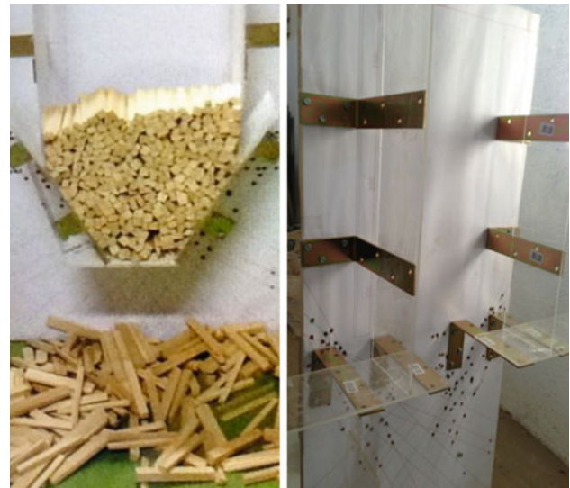
Fig. 1 Two-dimensional model silo. Front view ( left ), silo filled with wood particles and a hopper configuration; and side view ( right ), silo empty of particles and a flat-bottom silo configuration
