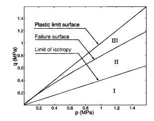
FIG. 16. Elastoplastic regimes: isotropic (I), anisotropic (II), and unstable (III).
