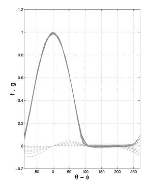
FIG. 13. Plastic profiles  $f(\theta)$  (solid line) and  $g(\theta)$  (dashed line). The results for different stress values have been superposed.
