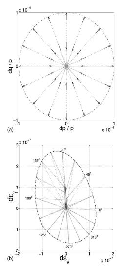
FIG. 6. Stress-strain relation resulting from the load-unload test. Dotted lines represent the paths in the stress and strain spaces. The dash-dotted line gives the strain envelope response and the solid line is the plastic envelope response.
