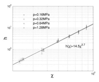
FIG. 15. Plastic modulus. The solid line is a power law fit with respect to the variable  $\chi = 1 - (p/p_0)^{\vartheta} q/q_0$ .
