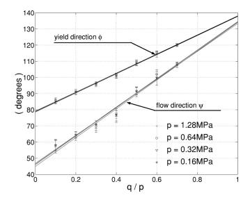
FIG. 14. The flow direction and the yield direction of the plastic response. Solid lines represent a linear fit.
