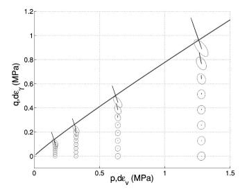
FIG. 7. Elastic response  $d\tilde{\epsilon}^e$  and plastic response  $d\tilde{\epsilon}^p$  resulting from the application of different loading modes with  $|d\tilde{\sigma}| = 10^{-4}p$ . The solid line represents the failure surface.
