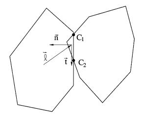
FIG. 1. Contact surface as defined from the geometry of overlap.
