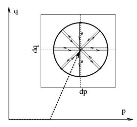
FIG. 4. Procedure to obtain the constitutive behavior: (1) The sample is driven to the stress state  $\tilde{\sigma}$ , with pressure *p* and shear stress *q*. (2) It is loaded from  $\tilde{\sigma}$  to  $\tilde{\sigma} + d\tilde{\sigma}$ . (3) It is unloaded to the original stress state  $\tilde{\sigma}$ .
