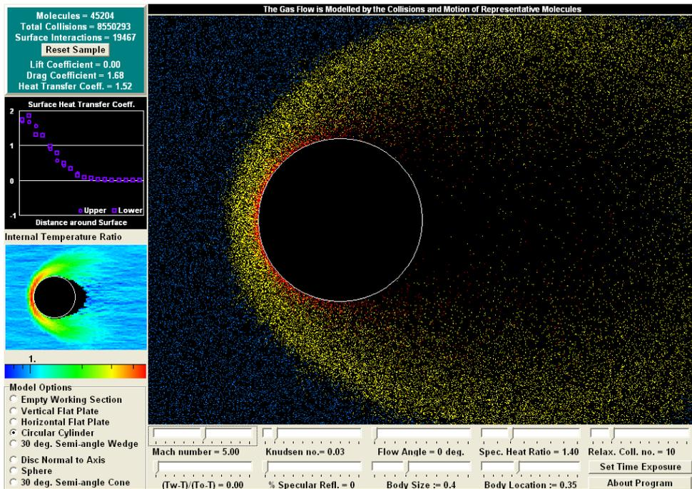
Figure 3.1: A virtual wind tunnel program using DSMC method, computing details of the flow field (e.g. pressure, temperature or velocities) around an object of arbitrary shape [1].
