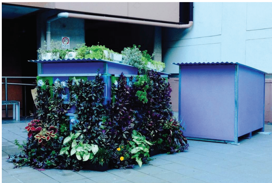
FIGURE 1. Green roof and green walls experimental setup.
