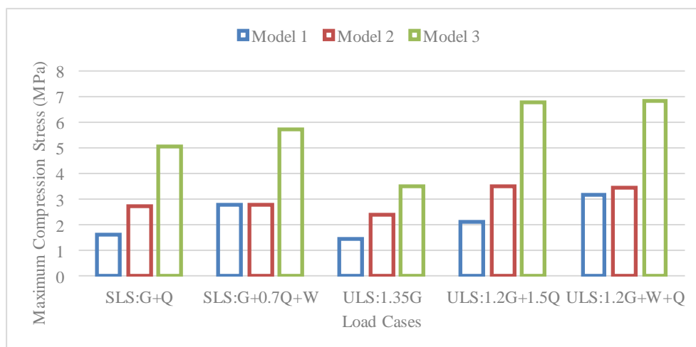
Figure 11. Summary of maximum compression stress for differing load cases and designs.
