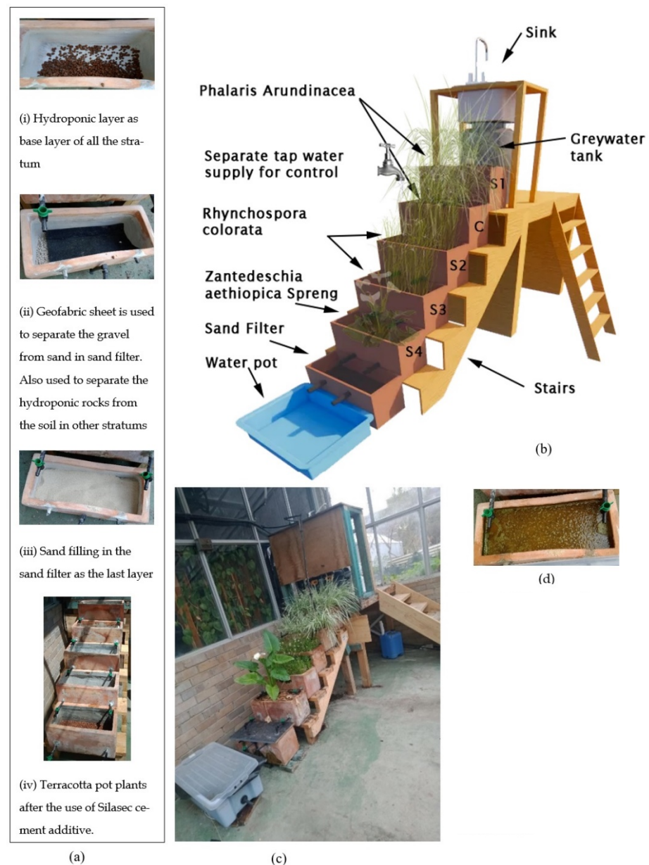
Figure 3. (a) Preparing the terracotta pot plants by arranging the substrate layers. (b) Three-dimensional model of the experiment, showing all the strata and their respective plant species ( Phalaris arundinacea in S1 and C, Rhynchospora colorata H. Pfeiff in S2 and S4 and Zantedeschia aethiopica Spreng in S4). (c) Experimental set-up in the off-grid tech lab at The University of Sydney. (d) Developed biofilm layer (Schmutzdecke) in the sand filter.
