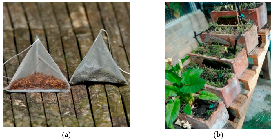
Figure 5. (a) Tetrahedron-shaped synthetic tea bags used for tea bag index (TBI) experiments: rooibos tea (left) and green tea (right). (b) Yellow stacks placed on the top of tea bag replicates of the planted areas. The main events of the TBI experimental process are described below: Day 1: All replicates were weighed and planted in Strata 1, 2 and 5. Day 4: The t_4 replicates were taken out and stored in the refrigerator at 4 °C. Day 7: The t_7 replicates were taken out. To remove the wet soil and the moisture, the replicates were put in the oven for a week at 50 °C. Day 14: The replicates were taken out of the oven. The dry soil around the replicates was removed through desiccation, and their final weights were noted. Day 25: The t_{25} replicates were taken out of the soil and stored in the refrigerator. Day 35: The t_{35} replicates were taken out of the soil and placed in the oven alongside the t_{25} replicates for one week at 50 °C. Day 42: The t_{25} and t_{35} replicates were taken out of the oven. Day 246: The t_{246} replicates were taken out of the soil and then stored in the oven for 7 days before weighing their final weights. After desiccation, their final weights were noted.
